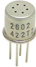
Figaro TGS2602 (sensitive to heavier VOCs)
