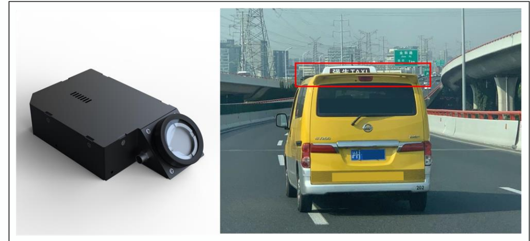
Figure 2. The mobile devices installed on a taxi's rear fins.
