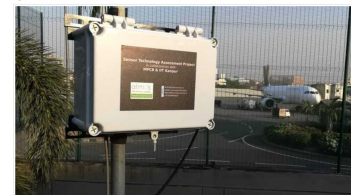
Low cost monitoring sensor network under an effort at scaling up light scattering technology using much smaller equipment as compared to existing air quality monitoring technology (AQI/PM2.5).
