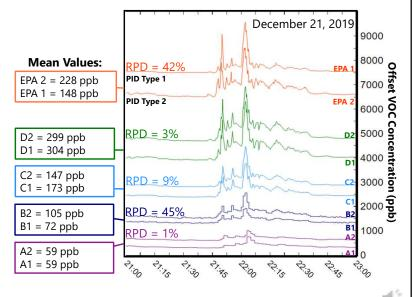
Simple single value offset only; EPA sensors rescaled to ppb and D Sensor Peak for comparison
