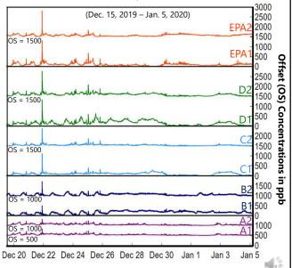
No fenceline-style baseline correction; single value offset used for best comparison; EPA sensors rescaled to ppb by D pair
