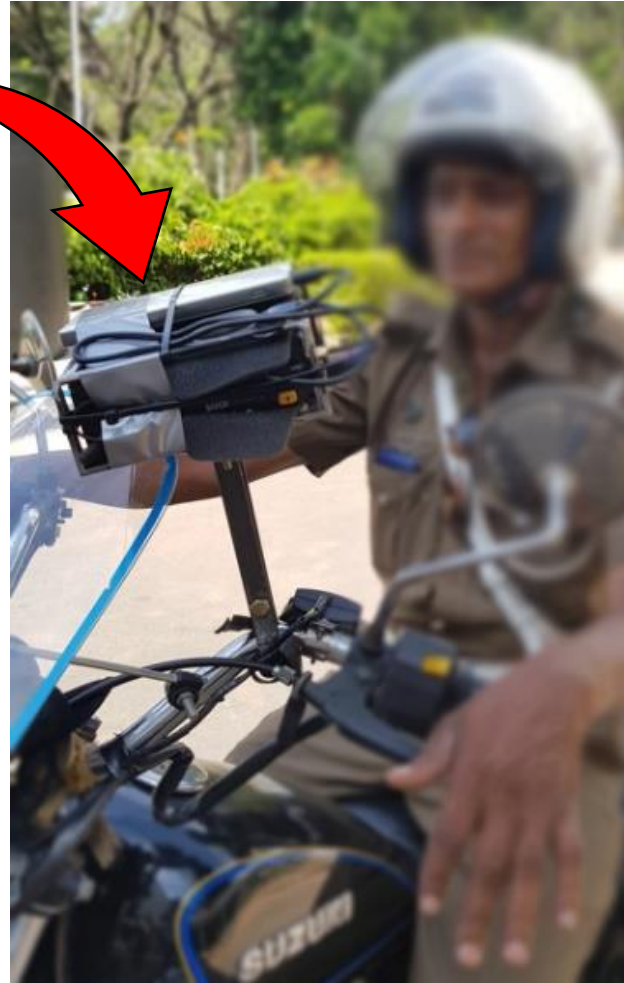
Fig 3. Sniffer 4D sensor mounted on a police traffic motorcycle
