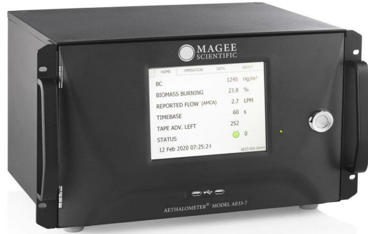
Black carbon monitor: Aethalometer
